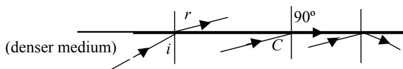
(i) total internal reflection occurs when the angle of incidence (in the more dense medium) is greater than the critical angle 3
